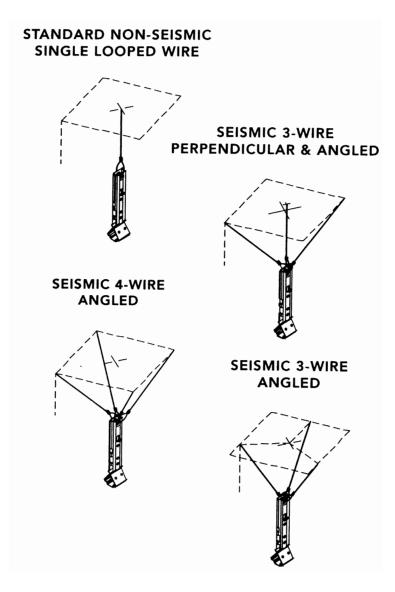
All top mounting brackets must be secured to the building structure. Shown are standard support configurations. Check with your local code authority as to which applies to your specific application.
