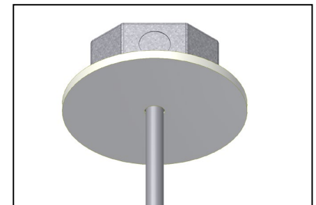
5. Twist the canopy clockwise onto the mounting strap to complete the installation.
