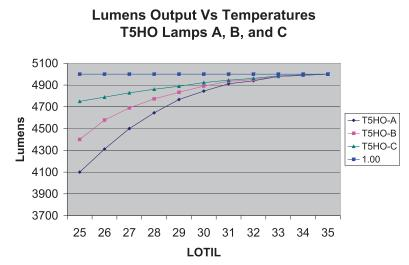
Fig. 3. Lumen Output vs Temperature of T5HO Lamps A B and C.
