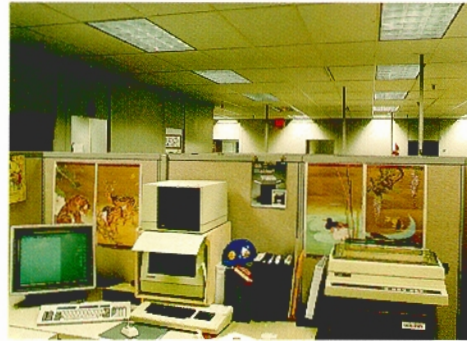
Open plan partitioned area with parabolic downlighting
