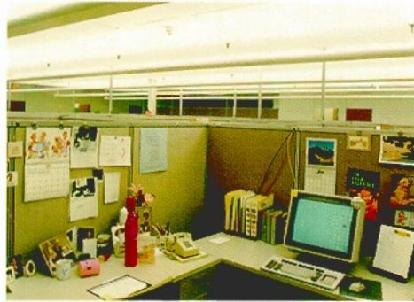
Open plan partitioned area with lensed indirect lighting
